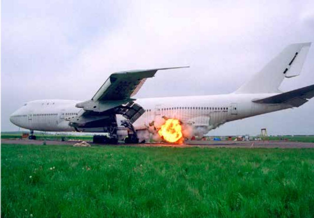
Boeing 747 undergoing cargo hold vulnerability testing at Aberdeen Proving Ground's Philips Army Airfield in Maryland.
