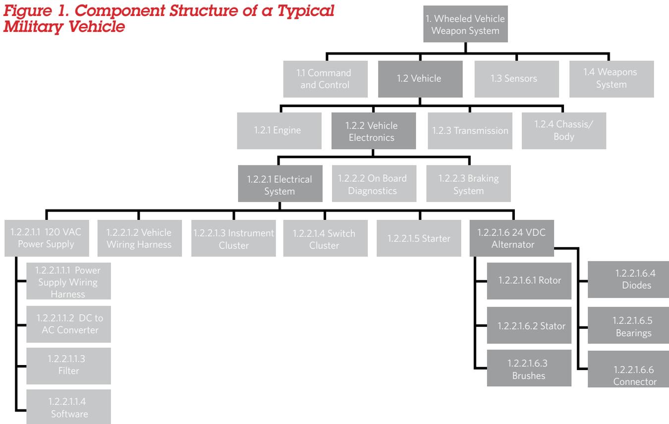
Our analysis starts with a description of a vehicle as a system with a specific architecture. Figure 1 is a partial Work Breakdown Structure (WBS) for a typical military vehicle, identifying the components of the major systems and illustrating the hierarchy among them. We assume that a family car would have a similar component structure.
